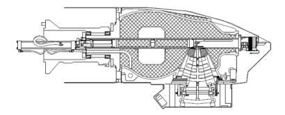
The design of the GammaBeam 100-80 head meets the international standards for source shielding, radiation transmission and radiation leakage. The dual control system monitors the source position and automatically retracts the source if a problem with source travel or position is detected. Operators and patients can feel confident that the GammaBeam 100-80 has been designed with their safety in mind.
